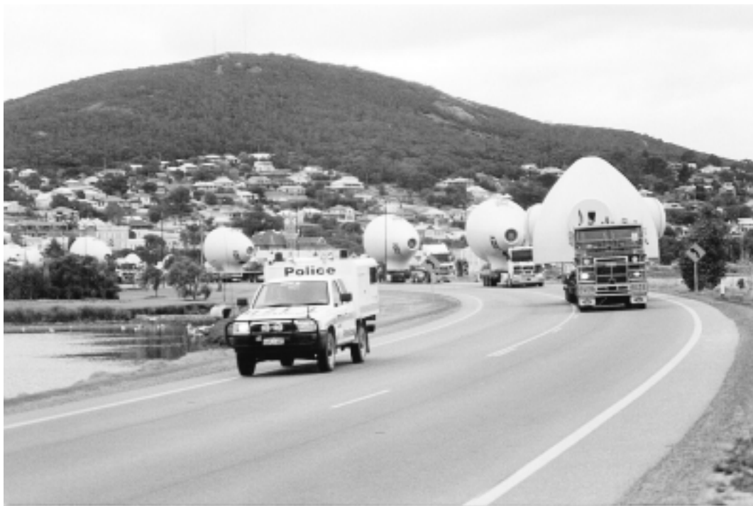
Figure 13 – Transportation of Nose Cones for 1.8 MW Wind Turbines for Albany Wind Farm (courtesy Western Power)
