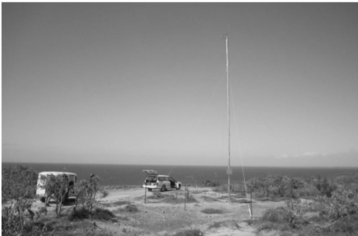
Figure 4 – 10m Pole Anemometry Mast (courtesy Aria Professional Services)
