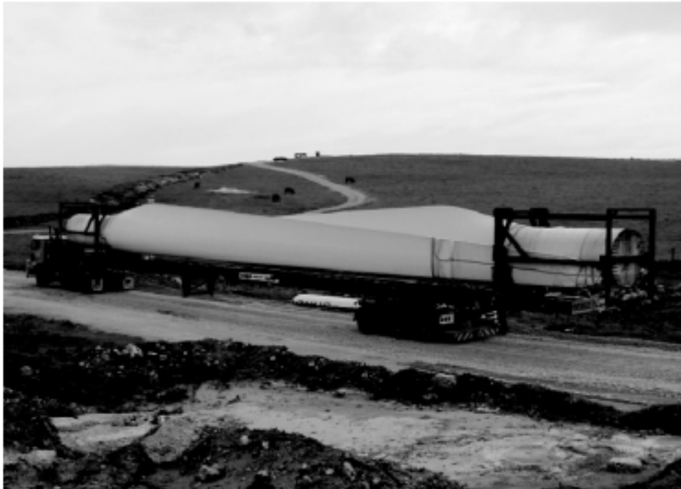
Figure 2 – Transport of Wind Turbine Blades On Site (courtesy Pacific Hydro)
