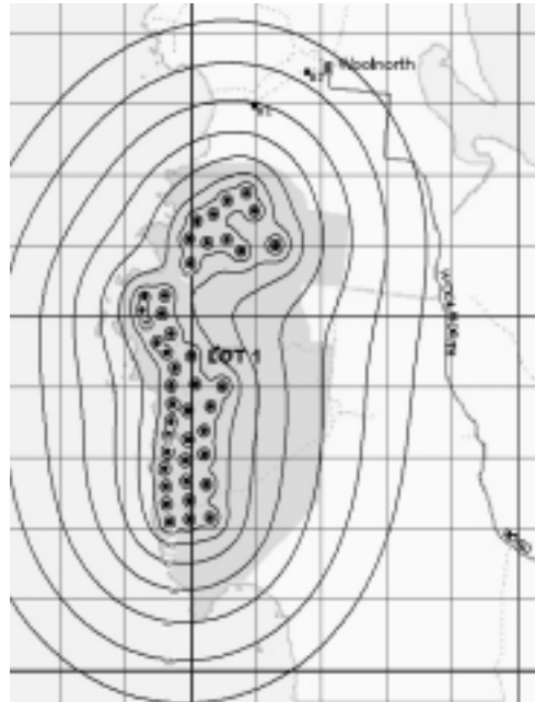
Figure 12 – Noise Contour Plot Showing Predicted Noise Levels at Residences (B1 & B2)(courtesy HydroTasmania)
