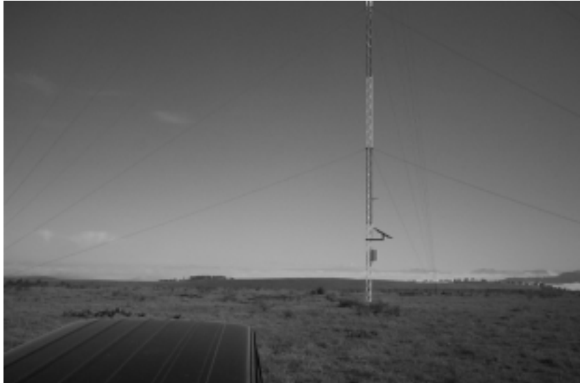
Figure 7 – Lower Section of 45 m Lattice Tower Anemometry Mast (courtesy Aria Professional Services)
